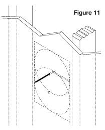
in a complete circle. If it turns freely, repeat the procedure from a hole about an inch above the center of your proposed speaker location (See Figure 11).
